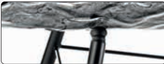
i Hinged beams at the upper side of the trestle can be adjusted individually to the shape of bowls and platters
